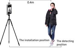
**2.3** After temperature detect are confirmed , make detect position mark on the ground for accurate detection.
